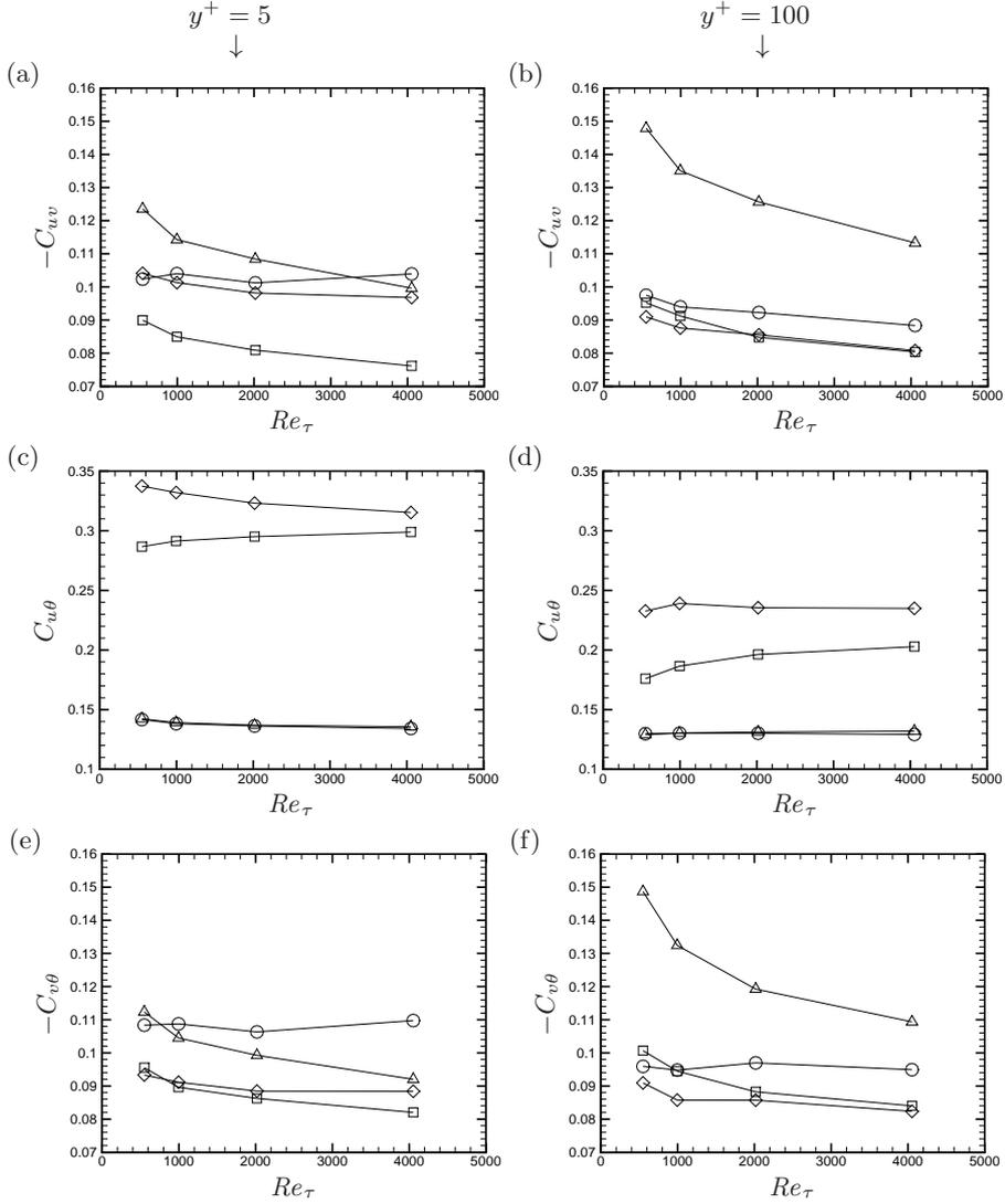
Figure 15: Quadrant contributions to correlation coefficients of  $u - v$  (a,b),  $u - \theta$  (c,d),  $v - \theta$  (e,f) at  $y^+ = 5$  (a,c,e), and  $y^+ = 100$  (b,d,f), for scalar field C. Quadrant I: squares; quadrant II: triangles; quadrant III: diamonds; quadrant IV: circles.
