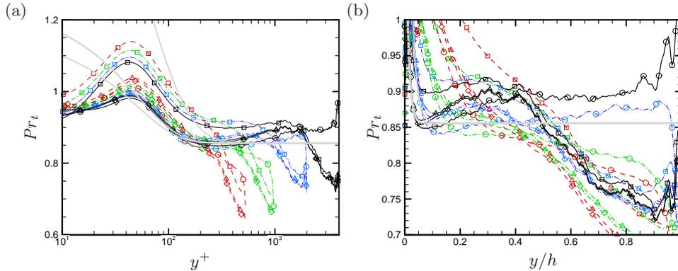
Figure 17: Turbulent Prandtl number as a function of wall distance. The thick grey lines indicate the predictions of equation (3.19) at  $Pr = 0.2, 0.71, 1$ . Refer to table 1 for nomenclature of the DNS data.
