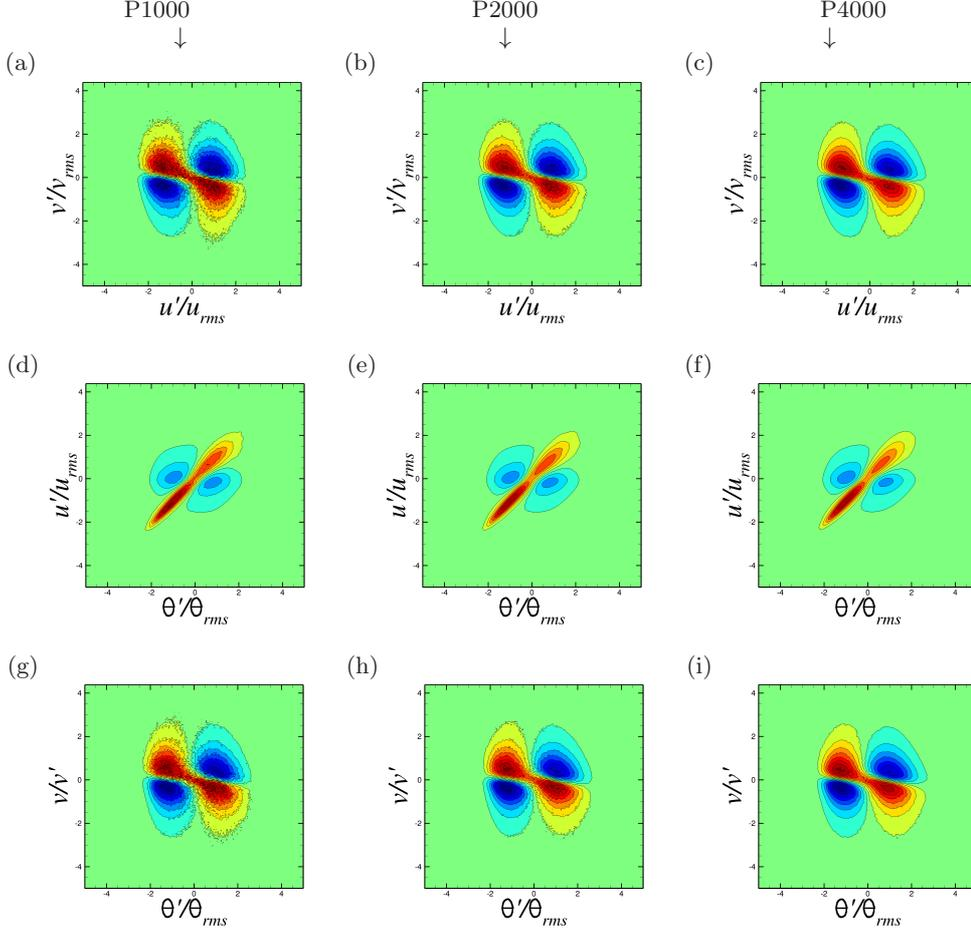
Figure 13: ‘Coherent’ part of joint pdfs at  $y^+ = 5$ , for flow case P1000 (a,d,g), P2000 (b,e,h), P4000 (c,g,i), scalar field C. Sixteen contour levels are shown, from  $-0.04$  to  $0.04$  in panels (a-c),(g-i) and from  $-0.36$  to  $0.36$  in panels (d-f). Colour scale is from blue (negative values) to red (positive values).
