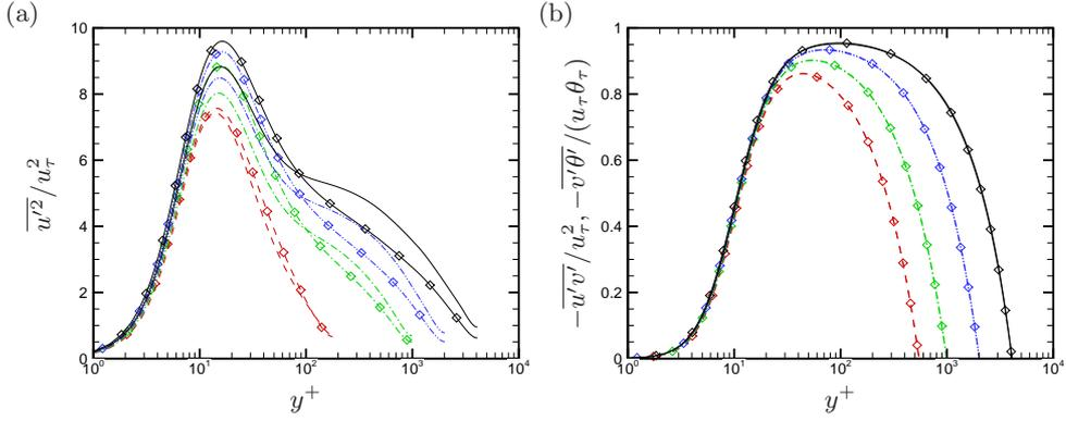
Figure 6: Variances (a) and vertical turbulent fluxes (b) for streamwise velocity field (lines) and passive scalar field C (lines+symbols). Refer to tables 1,2 for nomenclature.
