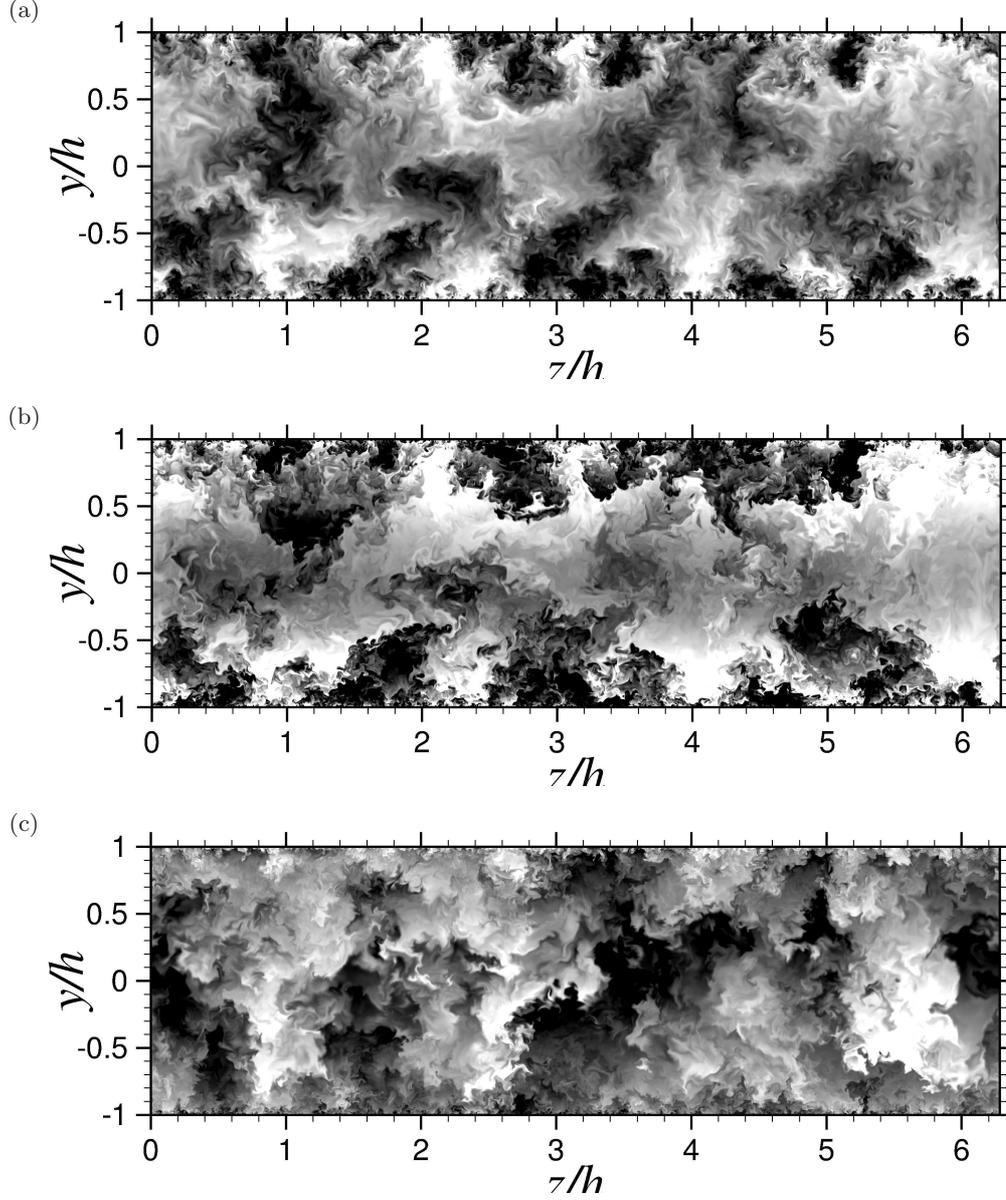
Figure 10: Instantaneous cross-stream visualizations of  $u'$  (a), and  $\theta'$  for scalar field C (b) and D (c), for flow case P4000. Panel (a): from  $-3u_\tau$  to  $3u_\tau$ ; panel (b): from  $-2\theta_\tau$  to  $2\theta_\tau$ ; from  $-4\theta_\tau$  to  $4\theta_\tau$ . Sixty-four contour levels are shown, in shades from black to white.
