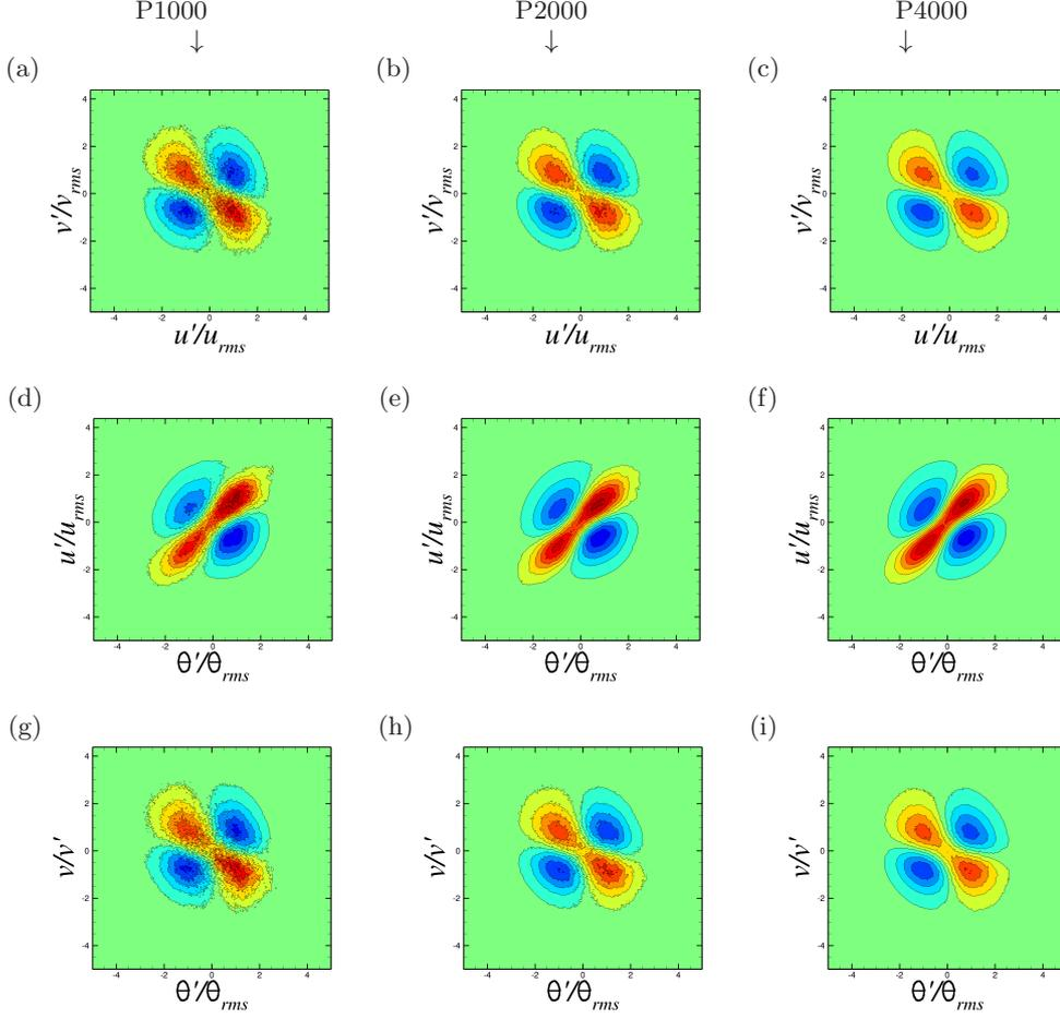
Figure 14: ‘Coherent’ part of joint pdfs at  $y^+ = 100$ , for flow case P1000 (a,d,g), P2000 (b,e,h), P4000 (c,g,i), scalar field C. Sixteen contour levels are shown, from  $-0.04$  to  $0.04$  in panels (a-c),(g-i), and from  $-0.1$  to  $0.1$  in panels (d-f). Colour scale is from blue (negative values) to red (positive values).
