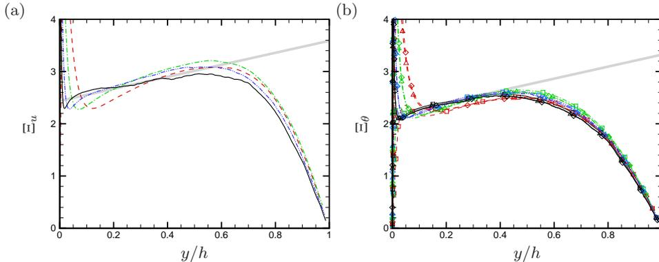
Figure 3: Diagnostic function for mean velocity (a) and for scalar fields A-C (b). The thick grey lines correspond to equation (3.8) with  $k = 0.41$ ,  $\gamma = 1.1$ ,  $\beta = 0$  (a), and  $k_\theta = 0.46$ ,  $\gamma_\theta = 1.15$ ,  $\beta_\theta = 0$  (b). Refer to tables 1,2 for nomenclature of the DNS data.
