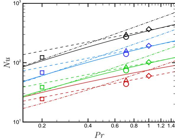
Figure 18: Nusselt number for scalar fields A-D (symbols as in table 2) at various Reynolds numbers (colors as in table 1), compared with the empirical formulas of Kays *et al.* (1980) (dashed lines), Sleicher & Rouse (1975) (dot-dashed lines) Gnielinski (1976) (solid lines).
