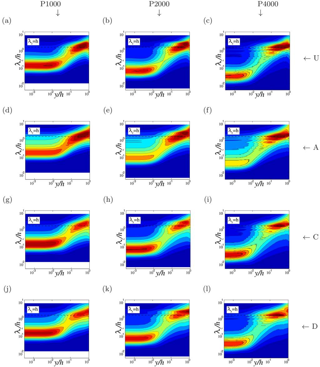
Figure 11: Variation of pre-multiplied, normalized spanwise spectral densities with wall distance: (a-c) spectra of  $u$  ( $k_z \hat{E}_u$ ) for flow cases P1000 (a), P2000 (b), P4000 (c); (d-l) spectra of  $\theta$  ( $k_z \hat{E}_\theta$ ) for flow cases P1000 (d,g,j), P2000 (e,h,i), P4000 (f,i,l), for the scalar fields A (d-f), C (g-i), D (j-l). Contour levels from 0 to 0.5 are shown, in intervals of 0.04.
