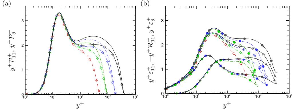
Figure 7: Pre-multiplied production (a) and dissipation rate (b) of streamwise velocity field (lines) and passive scalar field  $C$  (lines+open symbols). The solid symbols in panel (b) denote the contributions of viscous dissipation  $\varepsilon_{11}$  (squares) and pressure  $\mathcal{R}_{11}$  (diamonds), and their sum (circles). Refer to table 1 for the line style.
