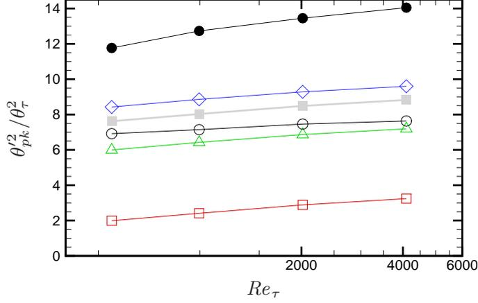
Figure 5: Peak scalar variances at various  $Pr$  (see table 2 for nomenclature of symbols) as a function of  $Re_\tau$ , compared with the peak streamwise velocity variance (solid squares). The solid circles denote the centerline peak of the scalar variance for field D.
